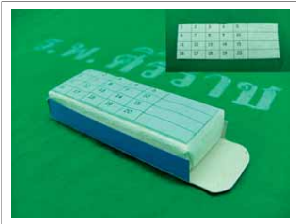
Fig 2. A table with 20 cells divided equally for the needles and leave 2 cm on the right side for the blade was placed on the front of wrapped floral foam.
